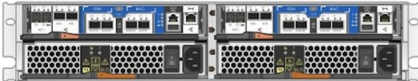
Figure 5) 10GBASE-T ports for connection through conventional RJ-45 Ethernet cables.
