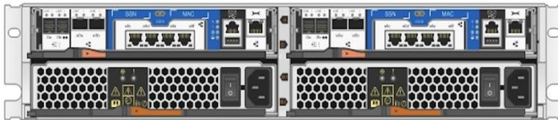
**Note:** For the 10GBASE-T port option, you must have a 10GBASE-T based uplink switch.
