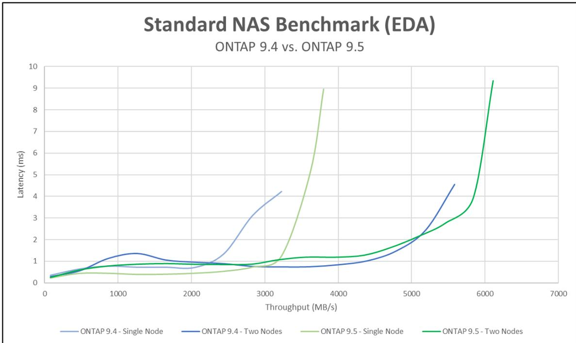
Figure 29 shows the performance for a standard NAS benchmark running a software build workload (such as Git or Perforce). Both types of workloads are ideal for FlexGroup volumes because of the high file ingest rates and need for parallel processing of write metadata.
