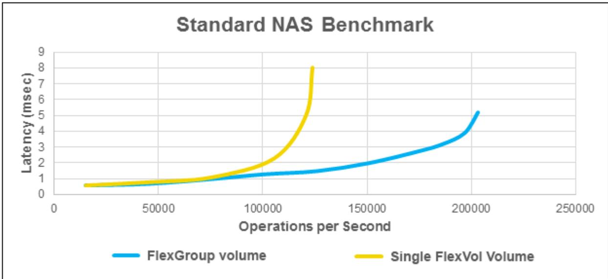
Figure 19 shows a performance comparison between a single FlexVol volume and a single FlexGroup volume. In a simple workload benchmark that used a software build tool (Git), a Linux kernel was compiled with the following hardware kit:
