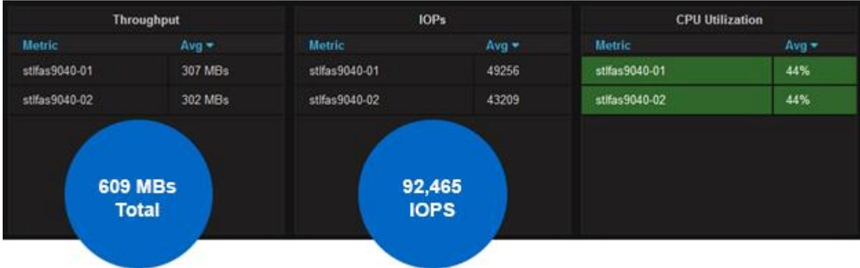
Figure 69) Average CPU utilization, throughput, and IOPS for a FlexGroup volume—single-node AFF A700, 128 threads.
