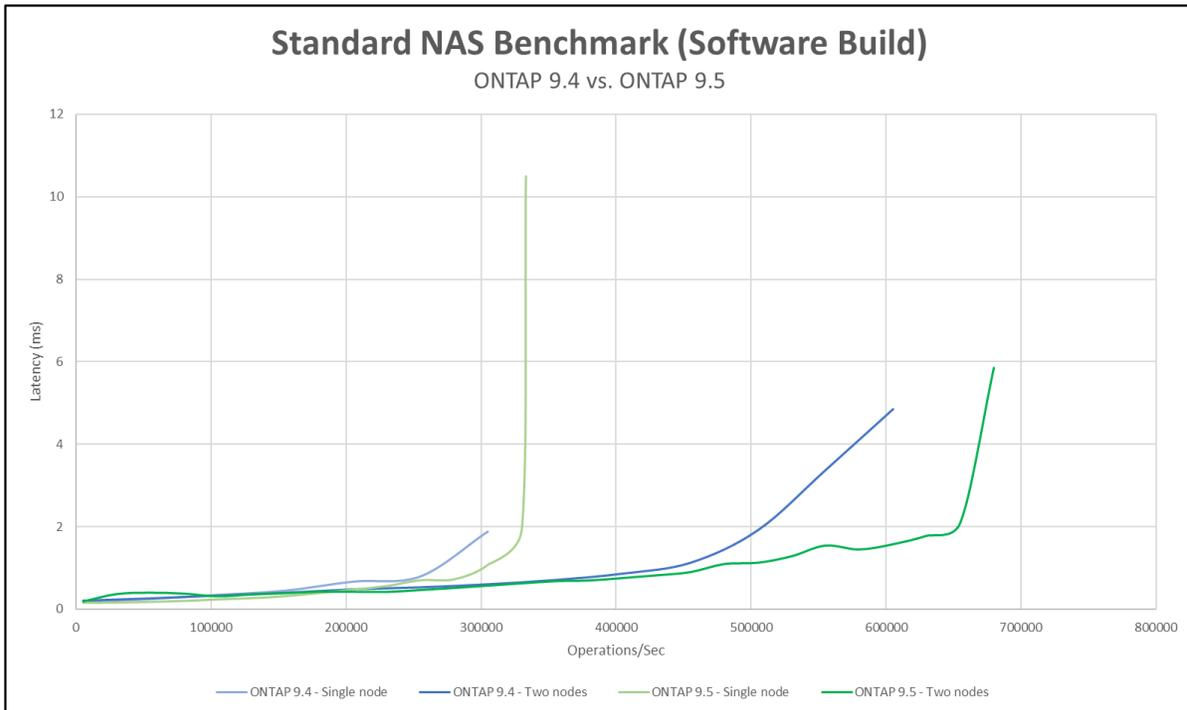
Figure 31) Standard NAS benchmark (software builds)—ONTAP 9.5 (MBps).
