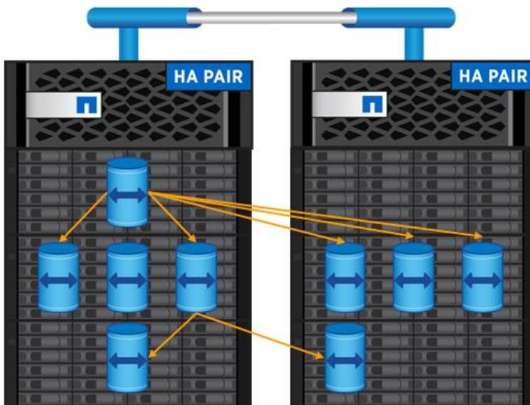
FlexVol volumes that are mounted to each other also do not provide true large buckets of storage, because each FlexVol volume is considered to be a folder in the file system to clients with 100TB limits. These folders also prevent the applications from controlling the narrative in file system layout. Instead, storage administrators must create the folder structure, forcing the application teams to reorganize their applications to fit into the folder constraints.
