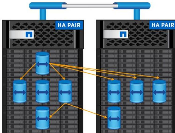
Although this architecture worked for many environments, it was awkward to manage and did not give a “single bucket” approach to the namespace, where the FlexVol volume’s capacity and file count constraints are limiting factors.
