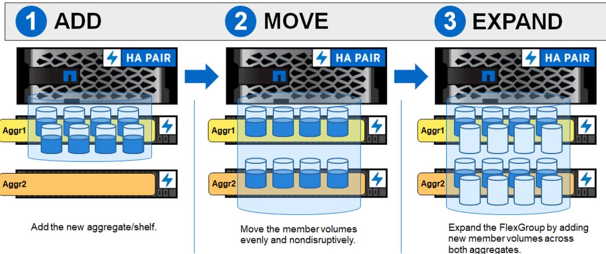
When adding new nodes to a cluster, follow the same steps for adding aggregates to a cluster. Use `volume move` and `volume expand` commands to adjust the member volumes.
