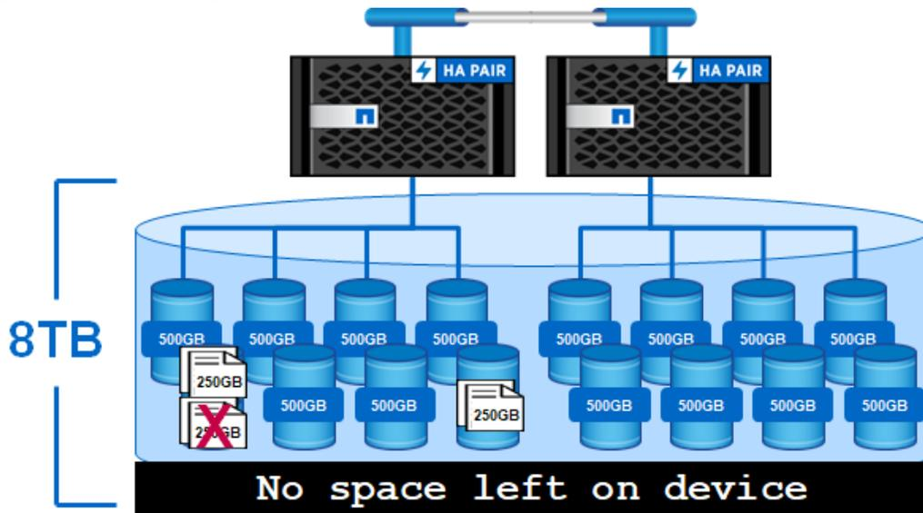
Features like volume autogrow (available starting in ONTAP 9.3) and [elastic sizing](#) (starting in ONTAP 9.6) can help offset the impact of this type of workload. Eventually, when physical space is exhausted, more storage must be added. Also, [adding nodes or disks](#) to a FlexGroup volume is nondisruptive, easy, and fast.
