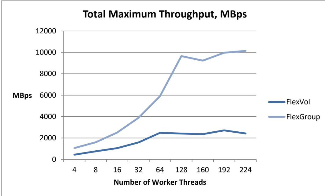
Figure 23 compares a FlexVol volume and a FlexGroup volume in the same configurations. This time, we break down the maximum read and write throughput individually, as well as comparing that against the average throughput for the FlexVol volume and the FlexGroup volume.
