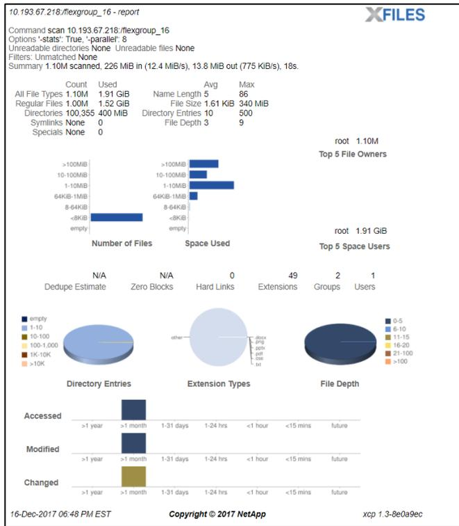
Using XCP to scan file systems provides average file size information, largest file size, capacity and file count measurements for the top five file owners, and much more. These statistics are available only in the NFS version of XCP, but you can still run NFS scans on datasets that only do SMB traffic by setting up a virtual machine that can use NFS.
