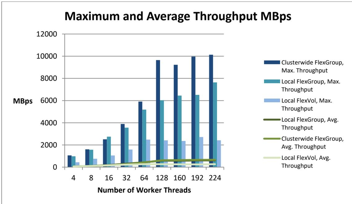
In Figure 65 and Figure 66, we compare read and write throughput, respectively, with the local and clusterwide FlexGroup volumes. At the 64-thread tipping point, the local FlexGroup volume starts to show a shift. Read throughput increases, while write throughput decreases. The cluster-wide FlexGroup volume shows the opposite trend.
