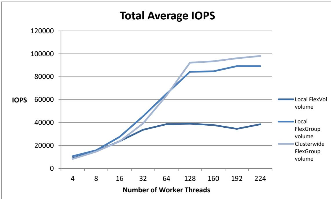
In this test, 64 worker threads appear to be a sweet spot. Let's look at the average CPU utilization for a single-node FlexGroup volume versus a FlexGroup volume that spans the HA pair at just above 64 threads. Keep in mind that using more CPUs is a good thing; it means that work is being performed. That work is evidenced by the greater number of IOPS and the higher throughput for a FlexGroup volume that spans multiple nodes under the same workload.
