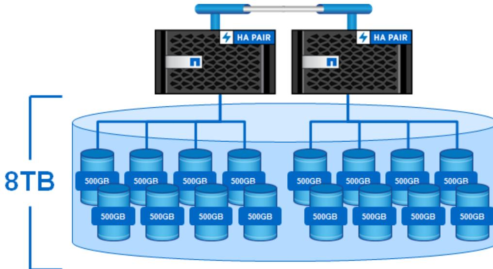
In many workloads, the distribution shown in Figure 45 would work well. However, if larger files in a workload would potentially fill in member volumes' large chunks of capacity used, then performance or even accessibility could be affected. Recall that if a member volume fills before other member volumes, the FlexGroup volume could report an “out of space” error in ONTAP versions earlier than 9.6.
