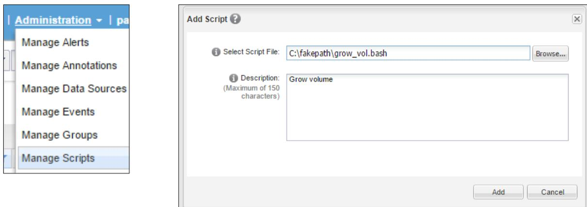
When the script is added to Active IQ, modify the alert to start the script when it is triggered. You can manage alerts through the Administration menu that is shown in Figure 103.
